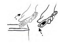
SECUNORM: high degree of safety thanks to the automatic blade retraction As with the fully automatic blade withdrawal, only you need to release the slider or lever during cutting.
